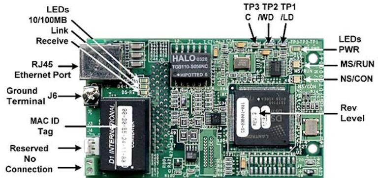
Connect to the *Modbus TCP/IP Option Card*.
