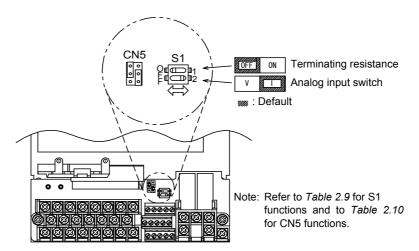
Fig 2.19 Shunt Connector CN5 and DIP Switch S1
