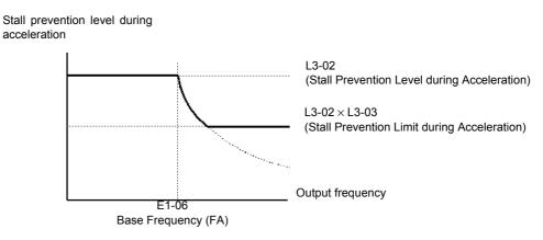
Fig 6.23 Stall Prevention Level and Limit during Acceleration
