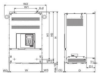
Fig 1.7 Exterior of enclosed, wall-mounted MxCs
