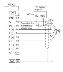
Fig 2.27 PG-X2 Connection Example (for a 12 V PG power supply)
