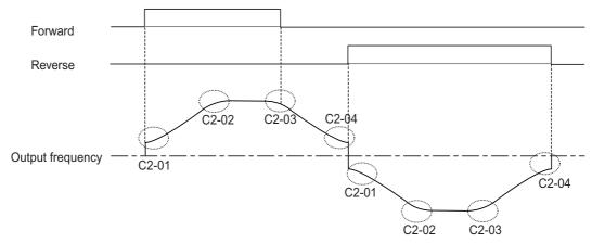
Fig 6.21 S-Curve Characteristic when Changing Motor Direction
