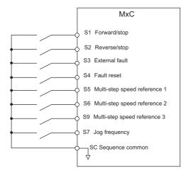
Fig 6.5 Control Circuit Terminal during 9-Step Operation
