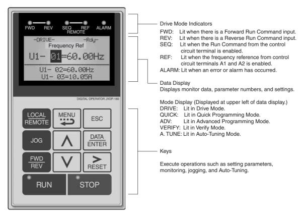
Fig 3.1 Digital Operator Component Names and Functions
