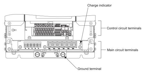
Fig 1.5 Terminal Arrangement (Model: CIMR-ACA4011)
