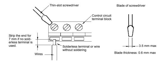
Fig 2.17 Connecting Wires to the Terminal Block
