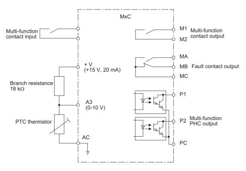
Fig 6.41 Mutual Connections During Motor Overheating Protection
