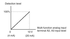
Fig 6.38 Overtorque/Undertorque Detection Level Using an Analog Input
