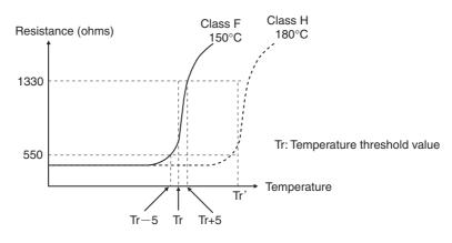
Fig 6.40 PTC Thermistor Temperature-Resistance Value Characteristics
