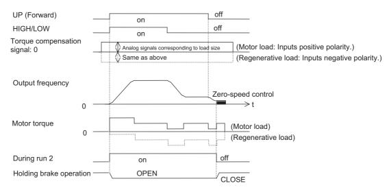
Fig 6.87 Torque Compensation Time Chart (Lifting)
