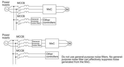
Fig 2.10 Incorrect Installation of a Power Supply Noise Filter
