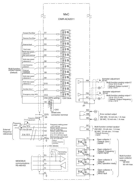
Fig 2.20 Control Circuit Terminal Connections
