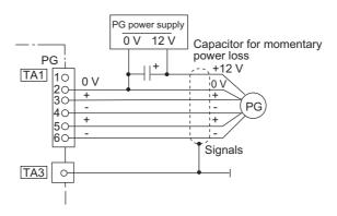
Fig 2.26 PG-B2 Connection Example
