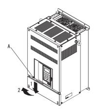
Fig 1.9 Removing the Terminal Cover (Model: CIMR-ACA4011)
