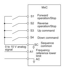
Fig 6.51 Connection Example when UP/DOWN Commands Are Allocated
