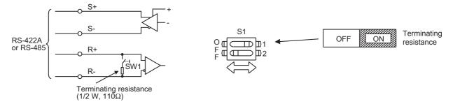
Fig 6.58 Communications Connection Terminal
