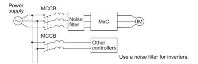
Fig 2.9 Correct Installation of a Power Supply Noise Filter
