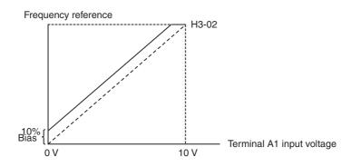
Fig 6.30 Example of Frequency Bias Adjustment
