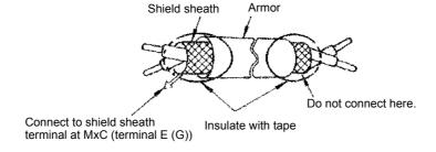
Fig 2.21 Processing the Ends of Shielded Twisted-Pair Cables
