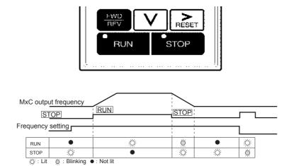
Fig 3.2 RUN and STOP Indicator LEDs
