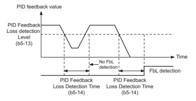
Fig 6.64 PID Feedback Loss Detection Time Chart
