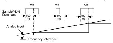
Fig 6.53 Sample/Hold Analog Frequency
