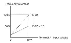
Fig 6.28 Example of Frequency Gain Adjustment
