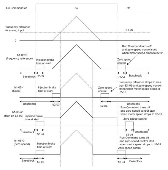
Fig 6.13 Decelerate to Stop (for Flux Vector Control)
