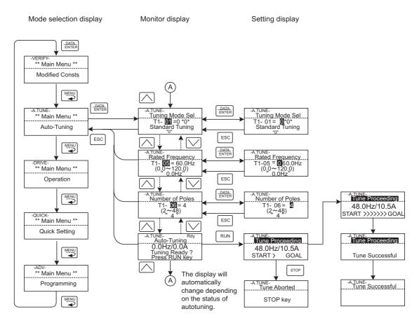
Fig 3.9 Screen Displays in the Auto-Tuning Mode
