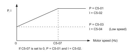
Fig 6.73 Low-Speed and High-Speed Gain Settings
