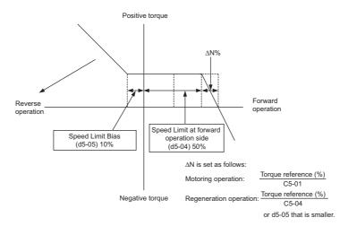
Fig 6.68 Speed Limit Bias Setting
