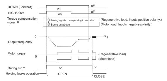
Fig 6.88 Torque Compensation Time Chart (Lowering)
