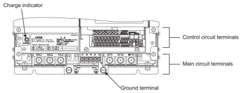
Fig 2.4 Terminal Arrangement (Model: CIMR-ACA4022)
