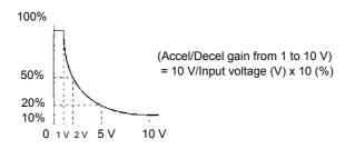
Fig 6.20 Accel/Decel Time Gain Using an Analog Input
