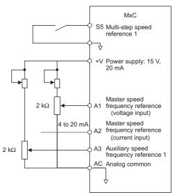
Fig 6.4 Switching between Master and Auxiliary Frequencies
