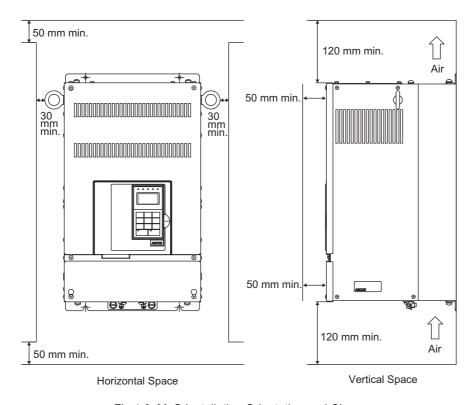
Fig 1.8 MxC Installation Orientation and Clearance
