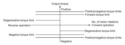
Fig 6.35 Torque Limit by Analog Input
