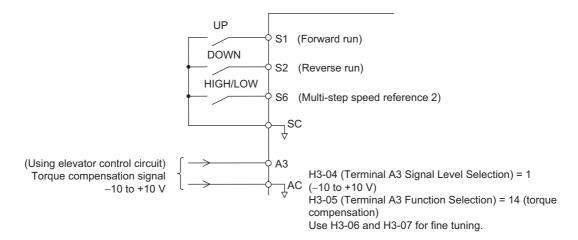
Fig 6.86 Torque Compensation Sequence Circuit Configuration
