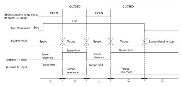
Fig 6.69 Speed/Torque Control Switching Time Chart.
