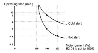
Fig 6.39 Motor Protection Operation Time
