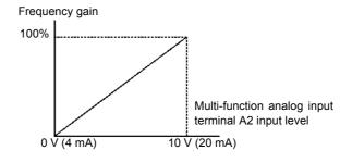
Fig 6.27 Frequency Gain Adjustment (Terminal A2 Input)
