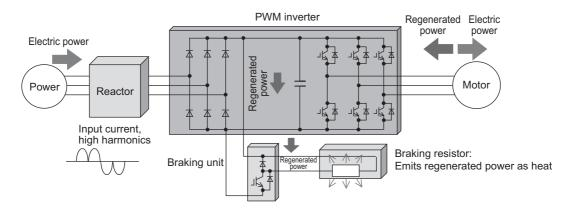
Conventional Type: Harmonic filter and power regeneration system with two external devices
