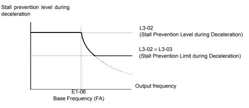
Fig 6.25 Stall Prevention Level and Limit during Deceleration
