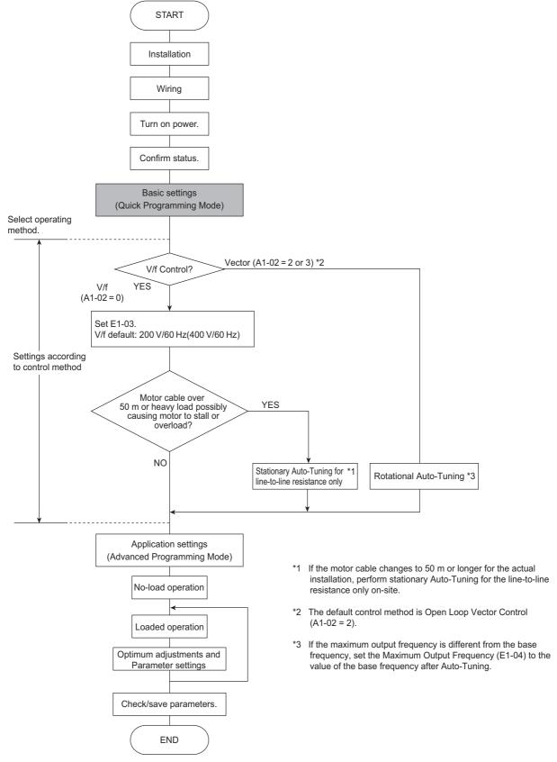
Fig 4.1 Test Run Flowchart
