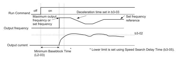
Fig 6.46 Speed Search at Startup (Using Current Detection)
