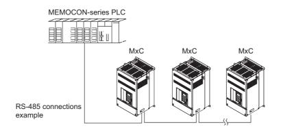
Fig 6.57 Example of Connections between PLC and MxC
