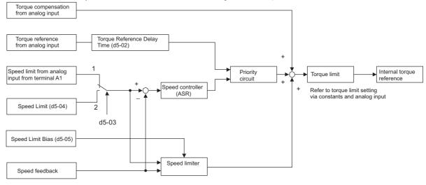
Fig 6.67 Torque Control Block Diagram
