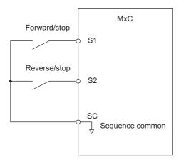
Fig 6.9 2-wire Sequence Wiring Example
