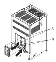
Fig 1.12 Mounting the Digital Operator (Model: CIMR-ACA4011)
