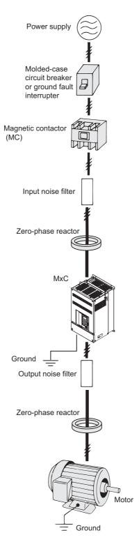
Fig 2.1 Example Connections to Peripheral Devices
