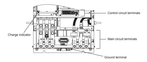
Fig 2.5 Terminal Arrangement (Model: CIMR-ACA2045)
