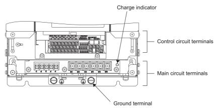
Fig 2.3 Terminal Arrangement (Model: CIMR-ACA4011)
