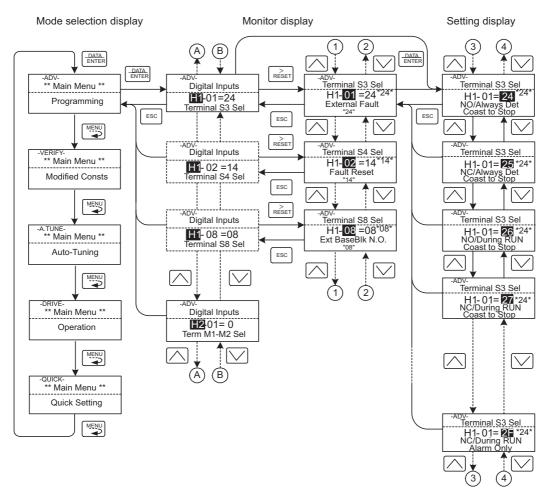
Fig 3.7 External Fault Function Setting Example
