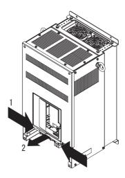
Fig 1.11 Removing the Front Cover (Model: CIMR-ACA4011)
