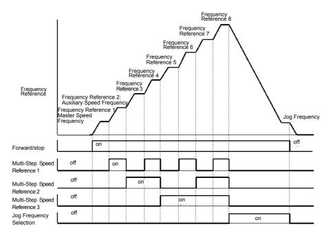
Fig 6.6 Multi-Step Speed Reference/Jog Frequency Selection Time Chart
