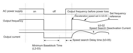
Fig 6.48 Speed Search After Baseblock (Current Detection: Loss Time > L2-03)
