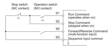
Fig 6.10 3-Wire Sequence Wiring Example
