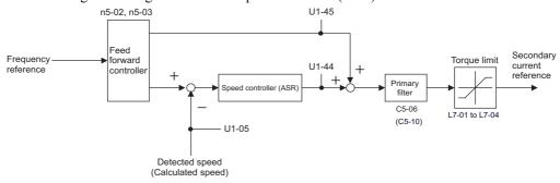
Fig 6.76 Structure of Speed Controller (ASR) and Feed Forward Control
