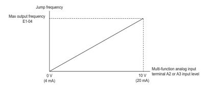
Fig 6.32 Jump Frequency Setting Using an Analog Input
