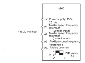
Fig 6.3 Current Input for Master Speed Frequency Reference
