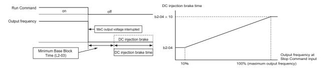
Fig 6.15 DC Injection Braking (DB) Stop
