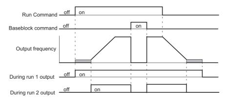
Fig 6.54 Timing Chart for "During Run" Output
