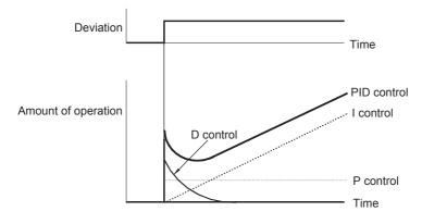
Fig 6.62 PID Control Operation
