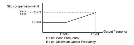
Fig 6.34 Slip Compensation Limit
