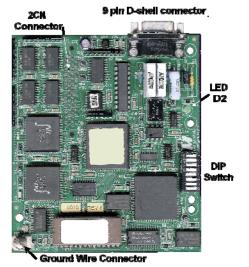
Apply power to the drive and verify that the diagnostic LED (D2) on the front of the Modbus Plus Option Card is in its correct state.
